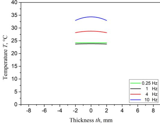
Figure 7 Temperature profile along the thickness of pure shear specimen of Material A. The tests were performed in displacement control with  $R\epsilon = 0.5$  with  $\epsilon_{\max} = 10\%$  at different frequencies.
