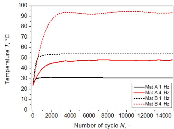
Figure 4 Temperature evolution of 3D dumbbell specimens for material A (black) and Material B (red). The tests were performed in force control with  $F_{\max} = 560$  N and  $R = 0.1$ , at frequency of 1 (full lines) and 4 Hz (dashed lines).
