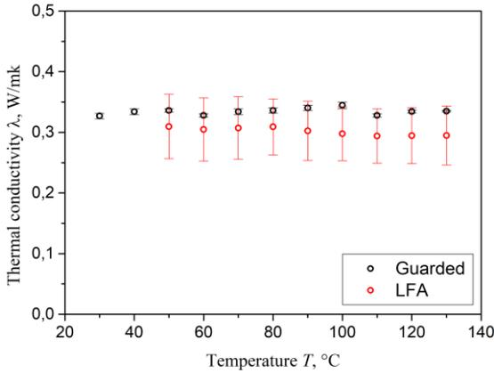
Figure 2 Values of thermal conductivity for Material B between 30 and 130 °C measured with two different techniques: in black the data obtained with the guarded heat method and in red the one obtained with the laser flash method.
