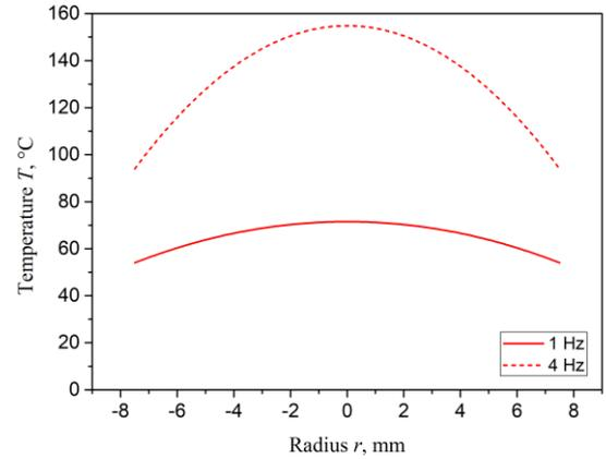
Figure 10 Temperature profile along the thickness of 3D dumbbell specimen of Material A. The tests were performed in force control with  $F_{\max} = 560\text{ N}$  and  $R = 0.1$ , at frequency of 1 and 4 Hz.
