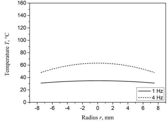
Figure 9 Temperature profile along the thickness of 3D dumbbell specimen of Material A. The tests were performed in force control with  $F_{\max} = 560\text{ N}$  and  $R = 0.1$ , at frequency of 1 and 4 Hz.
