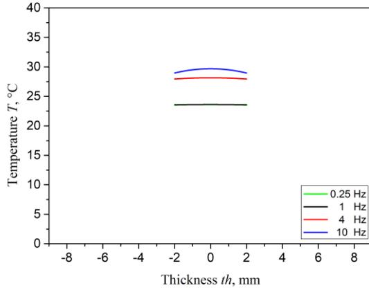
Figure 8 Temperature profile along the thickness of pure shear specimen of Material B. The tests were performed in displacement control with  $R\epsilon = 0.5$  with  $\epsilon_{\max} = 10\%$  at different frequencies.
